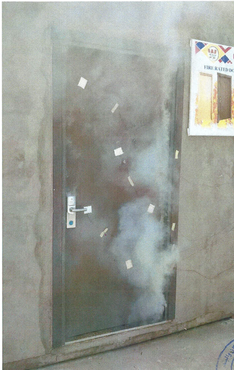
Figure (3): Smoke generation from the door during the first 04-10 minutes of test.
