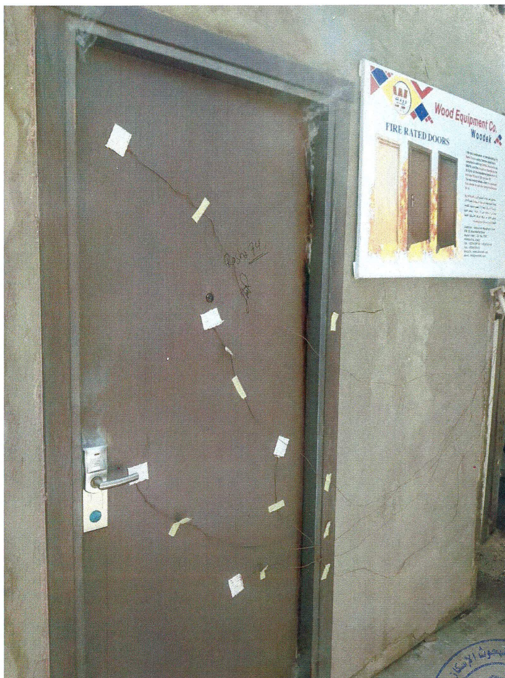
Figure (4): Photo of the unexposed surface of the door assembly at 30 th minute of test
