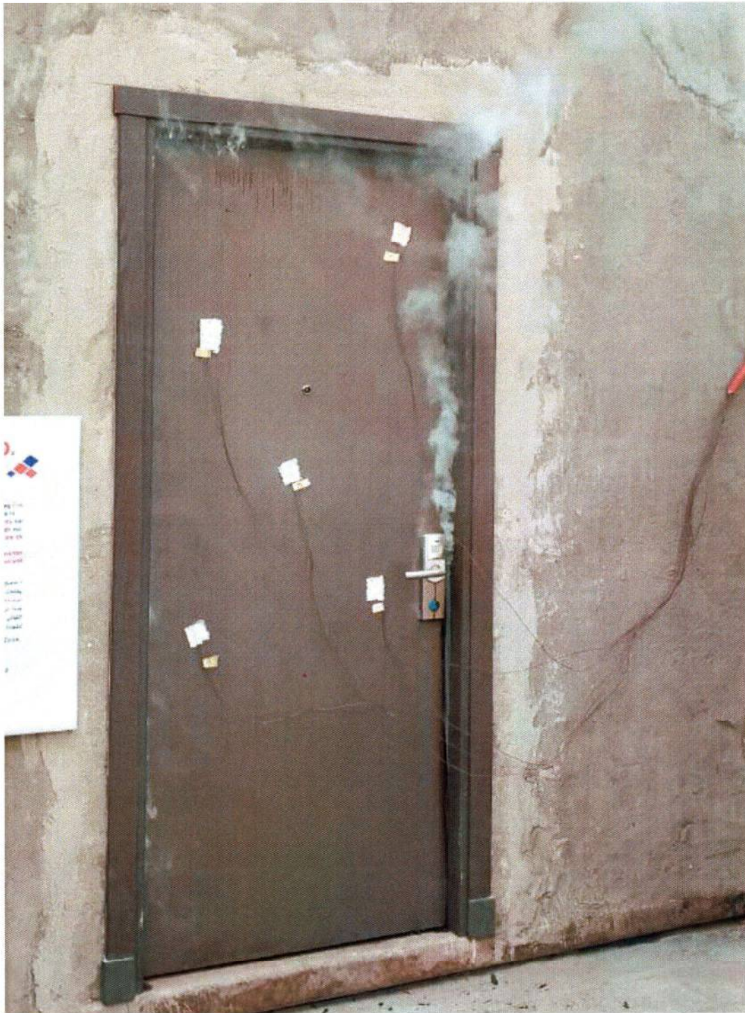
Figure (3): Smoke generation from the door during the first 10-15 minutes of test.
