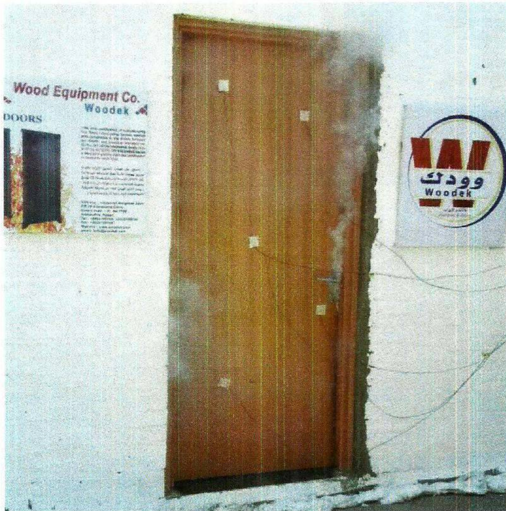
Figure (5): Heavy smoke was developed during the test.
