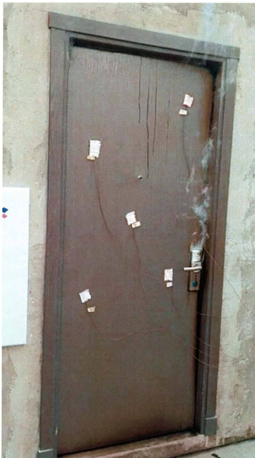
Figure (4): Photo of the unexposed surface of the door assembly at 30 th minute of test
